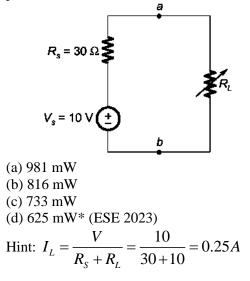
$$P = I_L^2 R_L = \left(\frac{1}{4}\right)^2 x_1 = 625 mW$$
