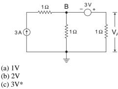
(d) 4V (SSC JE 2008) Hint: Apply KCL at node B  $\frac{V_B}{1} + \frac{V_B + 3}{1} = 3$ and  $V_A = 3x1$
