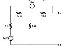
$\begin{array}{l} (a) \ 49.2 \ V, \ 10 \ \Omega \\ (b) \ -49.2 \ V, \ 15 \ \Omega \\ (c) \ -49.2 \ V, \ 20 \ \Omega^* \\ (d) \ 49.2 \ V, \ 20 \ \Omega \ (ESE \ 2024) \\ Hint: \ Applying \ KVL \ in \ loop \ 1 \\ 24 = 25I_1 + \ 30 \\ I_1 = -6/24 \ A \\ V_{th} = 5I_1 - \ 48 = 5(-6/24) - \ 48 = -49.2 \ V \\ R_{th} = [(10 + 10) \ \| \ 5] + \ 16 = \ 20 \ \Omega \end{array}$
