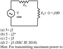
load in the circuit in question the value of source impedance must be equal to complex conjugate of load impedance. 247. Determine the maximum power (in W) transferred from the source to the load of the circuit given below:
