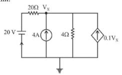
When supply by only 20V then current source is open circuit
