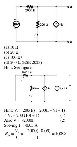
304. An experimental circuit as shown in the figure below has the variable resistor RL which is adjusted to the value of the load resistor as 10  $\Omega$ . What is the maximum load power?
