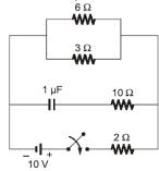
Hint: In steady state capacitor acts as an open circuit for DC supply.
