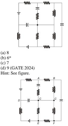
A point at which more than two elements are joints together is called Junction. A, B, C, D, E and F are junction.
