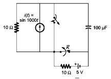
The switch K is closed and  $\overline{K}$  is opened simultaneously at the instant t = t<sub>1</sub>, where t<sub>1</sub> > 0. The minimum value of t<sub>1</sub> in milliseconds, such that there is no transient in the voltage across the 100 µF capacitor, is
