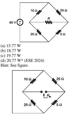
Condition for maximum power transfer is For  $R_{th}$  calculation,
