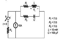
For time t < 0, the circuit is at steady state with the switch 'K in closed condition. If the switch is opened at t = 0, the value of the voltage across the inductor ( $V_L$ ) at t = 0<sup>+</sup> in volts is \_\_\_\_\_ (Round off to 1 decimal place). (GATE 2023) Hint: For t = 0<sup>-</sup>
