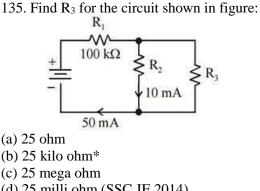
(c) 25 mega ohm (d) 25 milli ohm (SSC JE 2014) Hint: Apply KCL 50 mA = 10 mA + I I = 40 mA By current division rule Current in  $R_2 = 10$  mA =  $R_3/(R_3 + 1000 \text{ K}\Omega) \times 50$  mA
