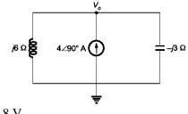
(a) -8 V (b) 8 V (c) 24 V\* (d) -24 V (ESE 2024) Hint: Applying KCL  $\frac{V_0}{j6} + \frac{V_0}{-j3} = 4 \angle 90^0$   $V_0 \left[ \frac{1}{j6} + \frac{1}{-j3} \right] = j4$  $\therefore V_0 = 24 V$
